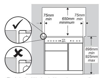
The hob should be level with, or above, any adjacent work surface. Above hob level a gap of 75mm should be left between each side of the cooker and any adjacent vertical surface. Surfaces above hob level at the sides and rear of the appliance should be heat, splash and steam resistant e.g. tiles.
